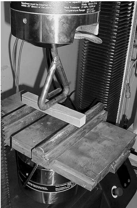
Fig. 5 Three-point flexural test apparatus
